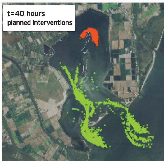
Figure 26: comparison of the current situation with foreseen interventions (sc.2). Simulation of particle transport of the semidiurnal sinusoidal tide oscillating between  $\pm 0.5$  m a.s.l. using the Lagrangian model.
