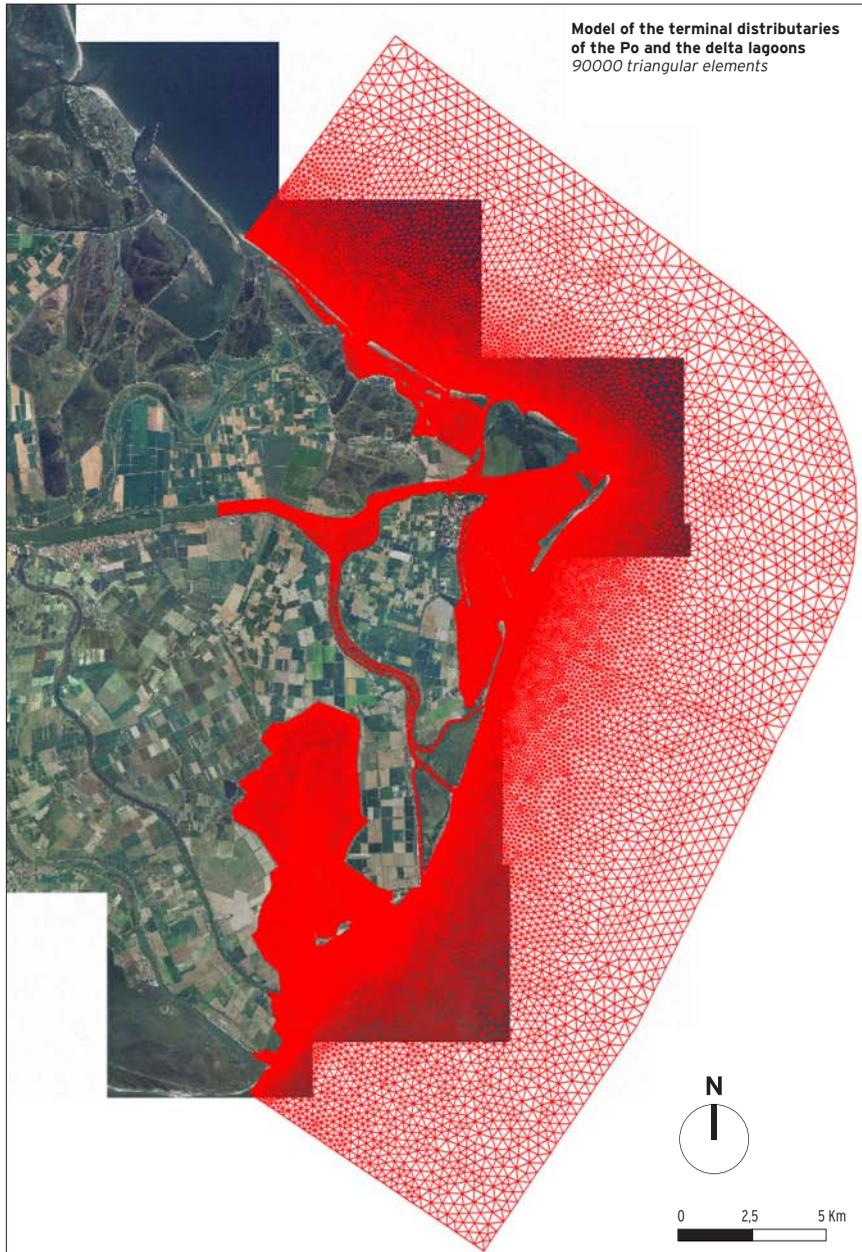
**Figure 30: two dimensional model of the terminal distributaries of the Po Delta, its lagoons and the stretch of sea (Matteotti/D'Alpaos - 2006 [11]) with the addition of the Sacca di Scardovari and the stretch of sea facing it.**
